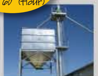
Example of installation with filling by bucket elevator
